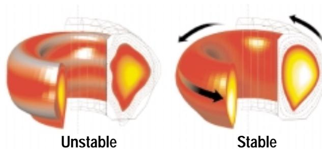
**Spinning plasma stabilizes the plasma surface allowing improved performance. Unstable kink mode distortion shown 10x exaggerated.**
