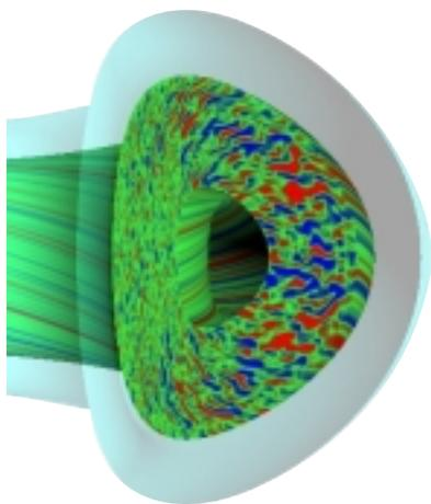
**Massively parallel computer calculations of turbulent electrostatic potential fluctuations are exhibiting the basic processes of plasma transport.**
