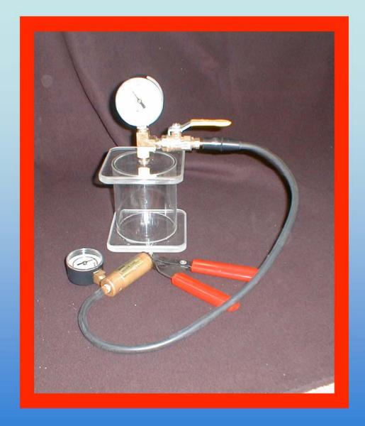
A completed vacuum chamber ready for a small balloon or marshmallow.
