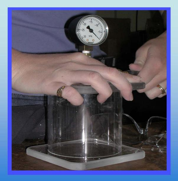
After the cylinder is glued to the base and the hardware is connected in the top, place an o-ring into the groove and place the top onto the cylinder. Attach the hand pump, evacuate, and leak check. Be sure the valve is in the open position for this step.
