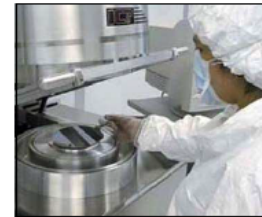
A technician prepares a plasma etcher, placing the wafer on the lower metal plate. In a large commercial manufacturing environment, the wafers are handled by robots, not humans.
